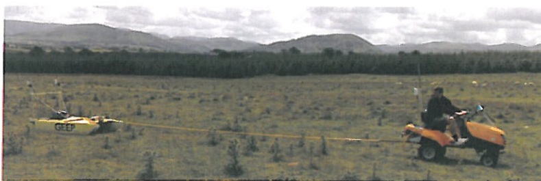
The collection of magnetic gradiometry data with dGPS location on foot or towed is an accurate and rapid means of data collection.
