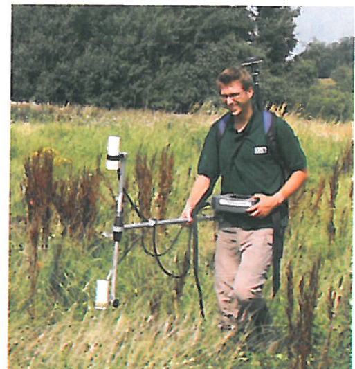
The collection of magnetic gradiometry data with dGPS location on foot or towed is an accurate and rapid means of data collection.
