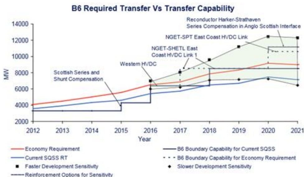
Figure 2.1 Reinforcement of the England-Scotland Transmission Boundary B6
