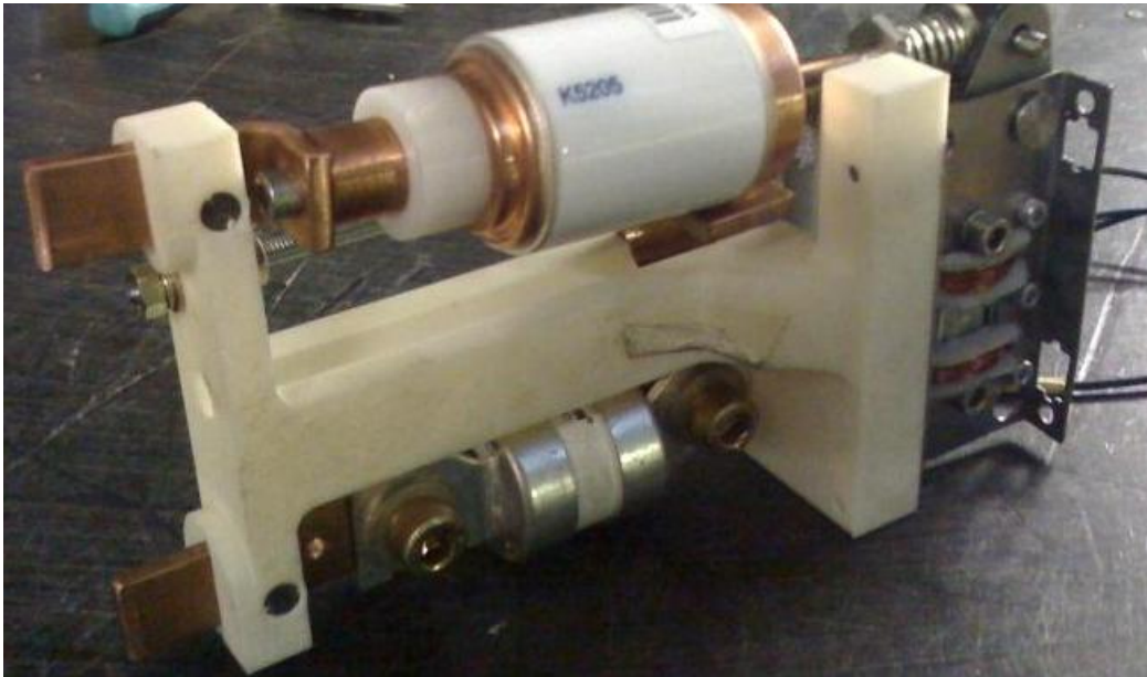
Figure 7-2 Prototype of the LV automation switch
