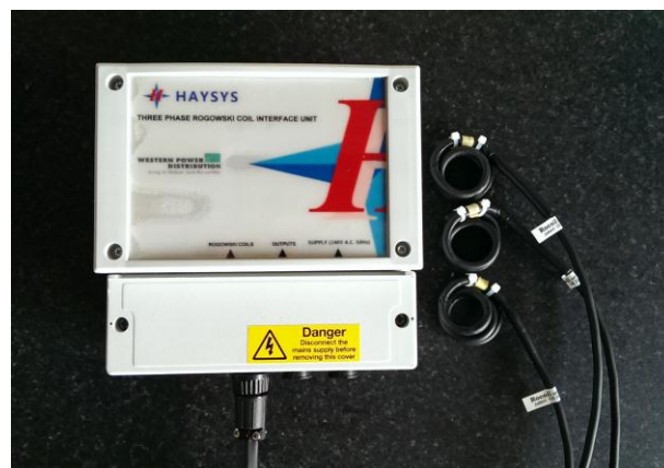
Figure 7 – Rogowski coil and transconductance amplifier Current transducer
