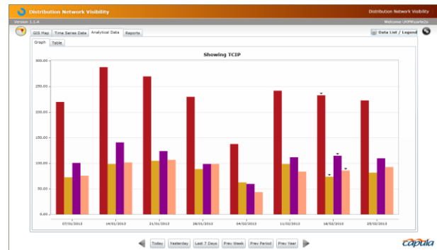
Analytical Tab: Bar Chart Data comparing the number of tap change operations of four primary Transformers
