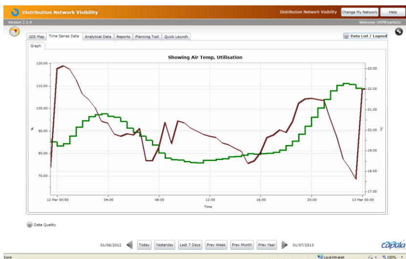
Figure F33: Half hourly average Air Temp and Utilisation for last 12 months. Peak Utilisation from Dec 12 to Mar 13 (winter) Air Temp: Green; Utilisation: Brown
