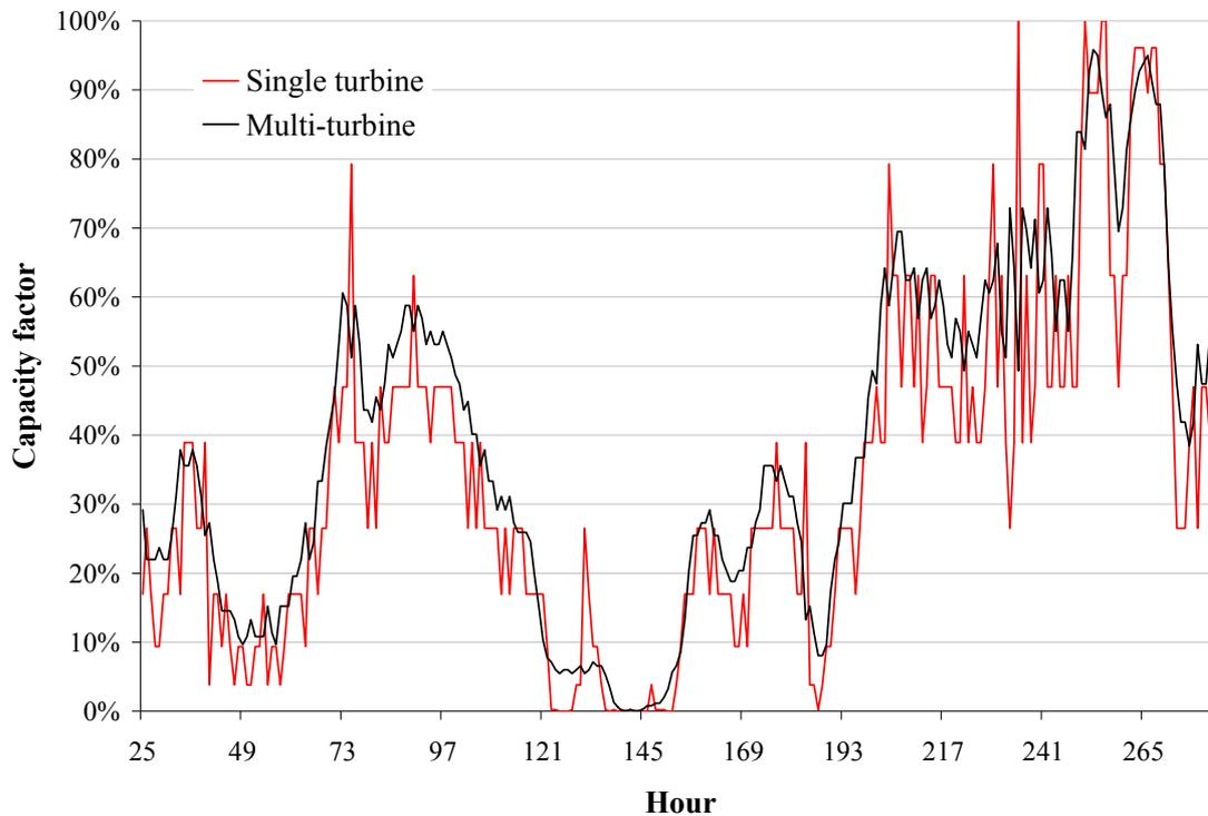
The next step is to calibrate the estimated wind output by comparing monthly average capacity factors from the multi-turbine approach to actual historic CFs. The CFs we estimate will be too low, because we are using wind speed measured from a weather mast, which is at a lower height (10 m) than the wind turbine (which will be at a height of over 30 m). Consequently the actual wind turbine will experience higher CFs than we estimate from our wind speed data.
