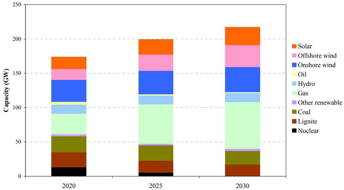
**Table 10: Installed capacity in Germany by scenario (GW)**
