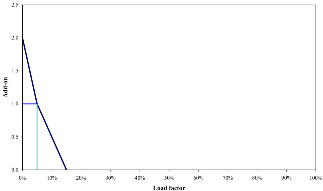
The shape of the fixed cost add-ons depends on the assumptions that are made regarding (i) the overall load factor for peaking plant - 15% in this example, (ii) the load factor at which the slope of the add-ons can change - 5% in the example and (iii) the relative scale of the add-ons at the absolute peak and the intermediate break point – 2:1 in the example.
