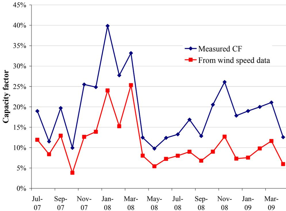
The final step is to characterise the time-series of electricity production for WPG in a way that we can model probabilistically. We do this by having a function that can generate a random series of CFs, which still respect average historic CFs and changes in a realistic way.
