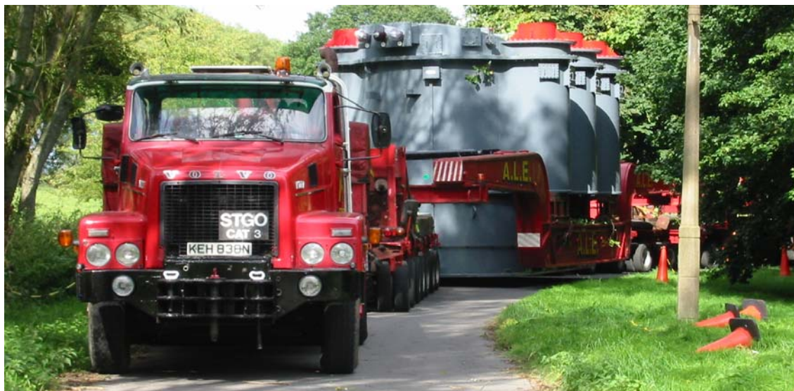
Figure 3. New Supergrid Transformer being transported to site
