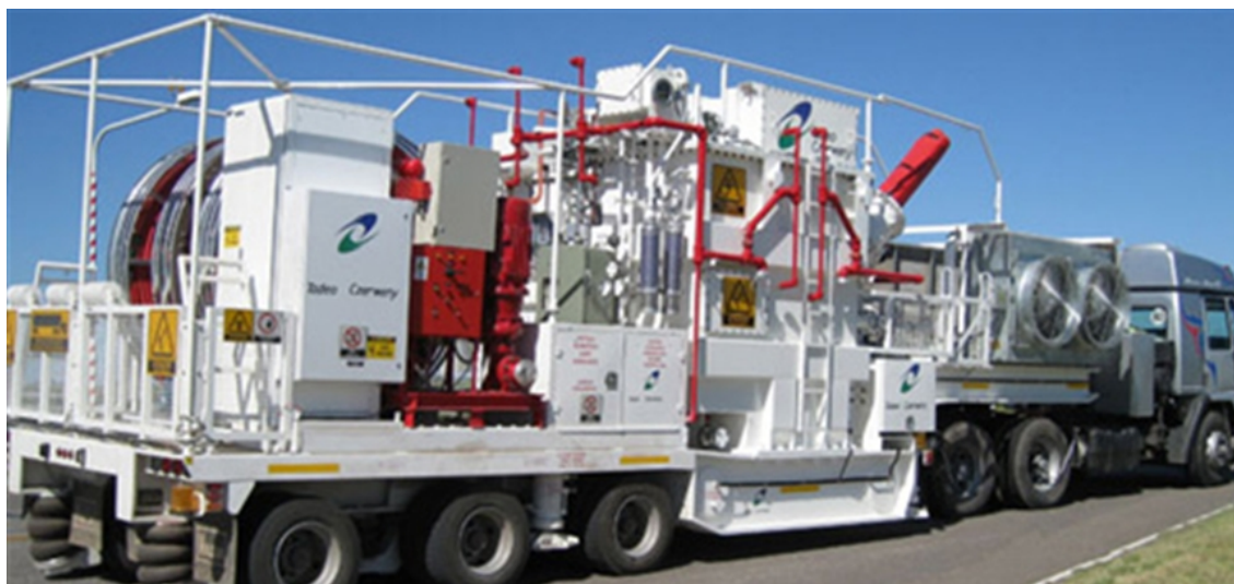
Figure 4. Example of a 132kV Mobile Transformer Transportation
