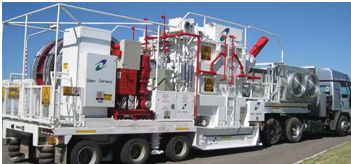
Figure 4. Example of a 132kV Mobile Transformer Transportation
