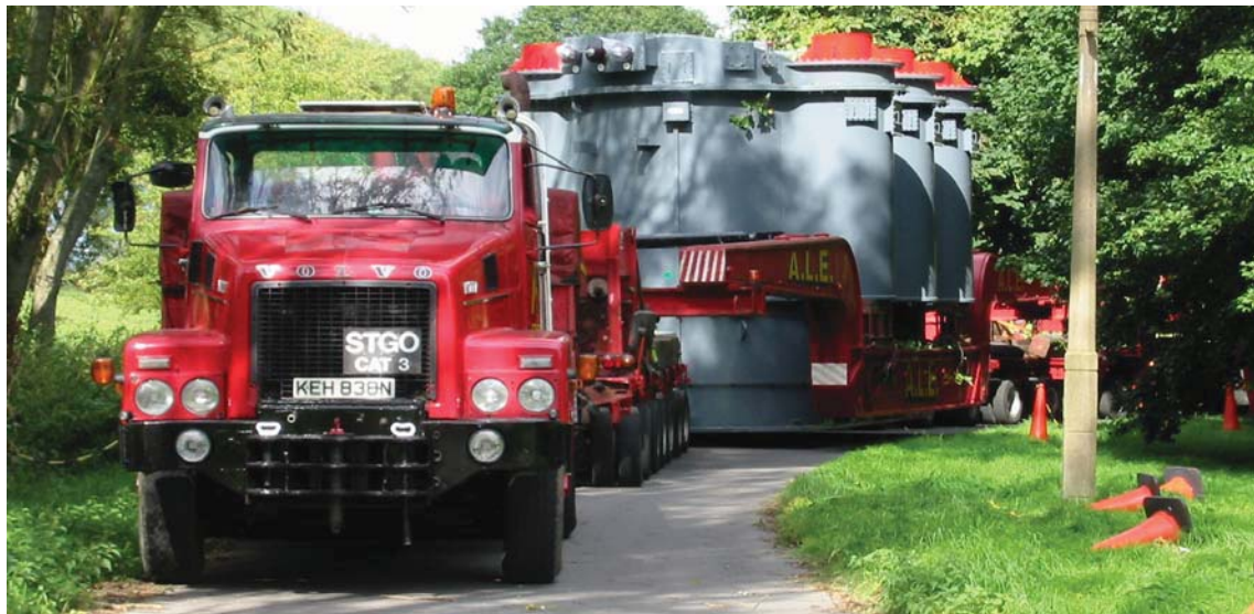
Figure 3. New Supergrid Transformer being transported to site
