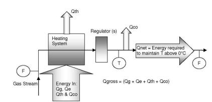
System efficiency,  $\eta$ , is defined by:  $\eta$  (%) =  $\frac{Qnet}{Qaross}$
