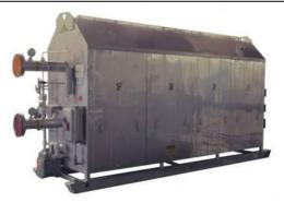
HotCat's are made up of several zones each containing 2 catalytic heaters. Each zone can be controlled independently. Bruest state in their literature that the efficiency of their system is 70%. However, this figure does not include electricity consumption. Before the gas supply is provided to each heater, the catalyst needs to be preheated to 232°C by an electrical preheating element. Once achieved, the electrical supply is disconnected and gas combusts to provide all of the required heat.
