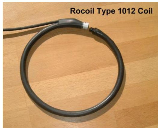
Figure 21: Haysys flexible Rogowski coil.
