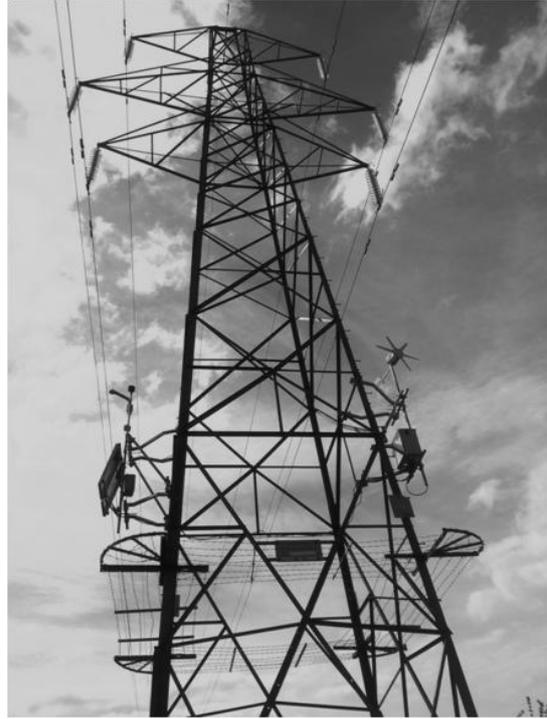
Figure 4-11: Tower-based weather station
