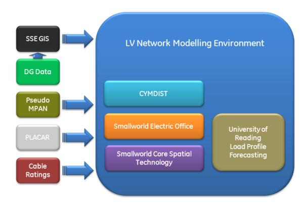
Figure 2 - Low Voltage Network Modelling Environment data sources and components
