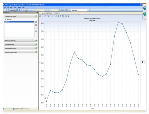
Figure 12 -CYMDIST – Energy Profile Manager – 24 Hour Profile load profile
