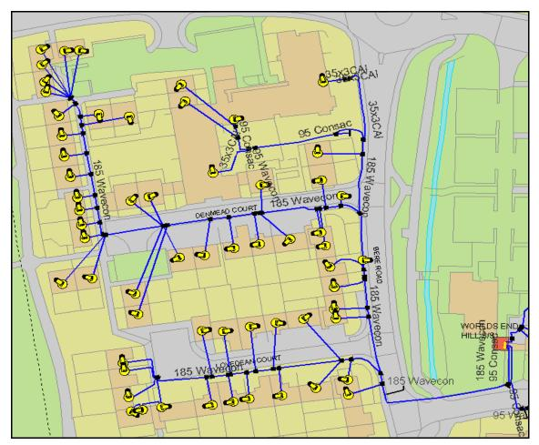
Figure 6 – The same area of SSEPD's low voltage network as shown in Fig. 5 migrated from GIS to Smallworld Electric Office
