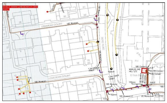
Figure 5 - Example of SSEPD's GIS system displaying a single substation, low voltage feeder cables and services
