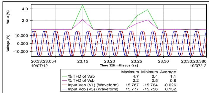
**Figure 4. THD with 20 Ω impedance**
