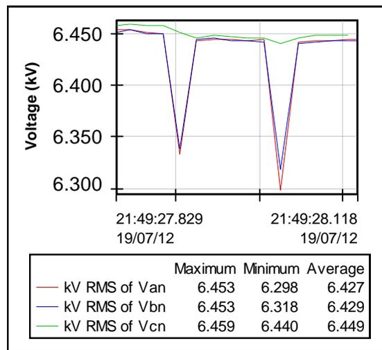
**Figure 2. Voltage fluctuation for FL 12.88kA and X/R 13.30**
