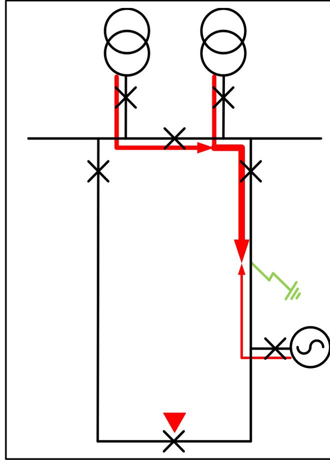
**b) Fault in-feed for solid configuration**
