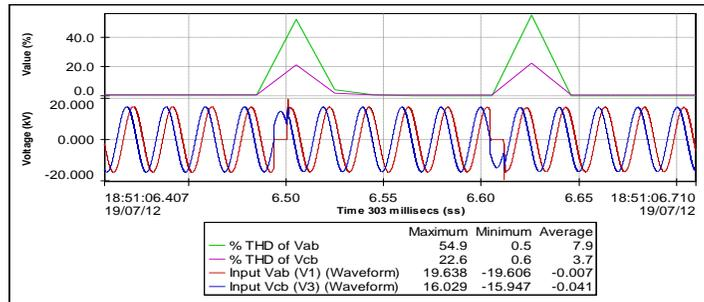
**Figure 3. THD with zero additional impedance**
