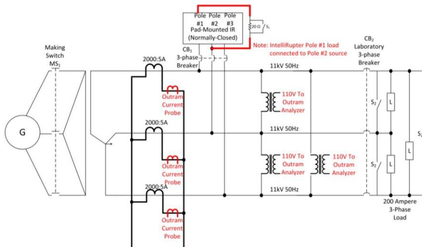
**Figure 1. Laboratory Test Set-Up**
