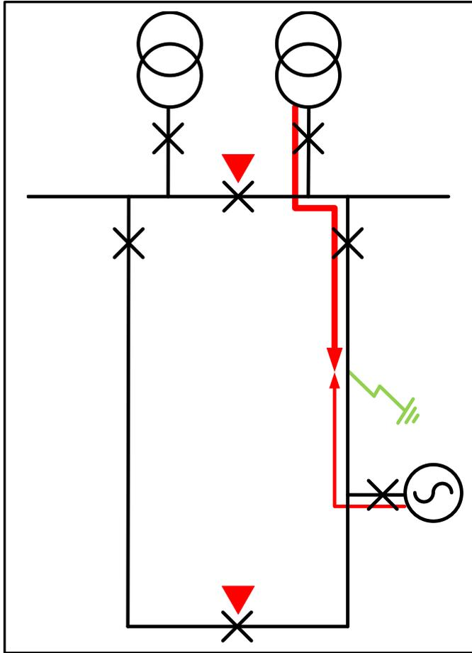
**a) Fault in-feed for split configuration**
