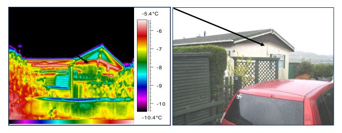
In the thermal image "pre-improvement", it is clear that significant heat loss is occurring across the building envelope and that this can be attributed to thermal bridging across the timber frame construction in addition to warm air leakage at critical junction details.
