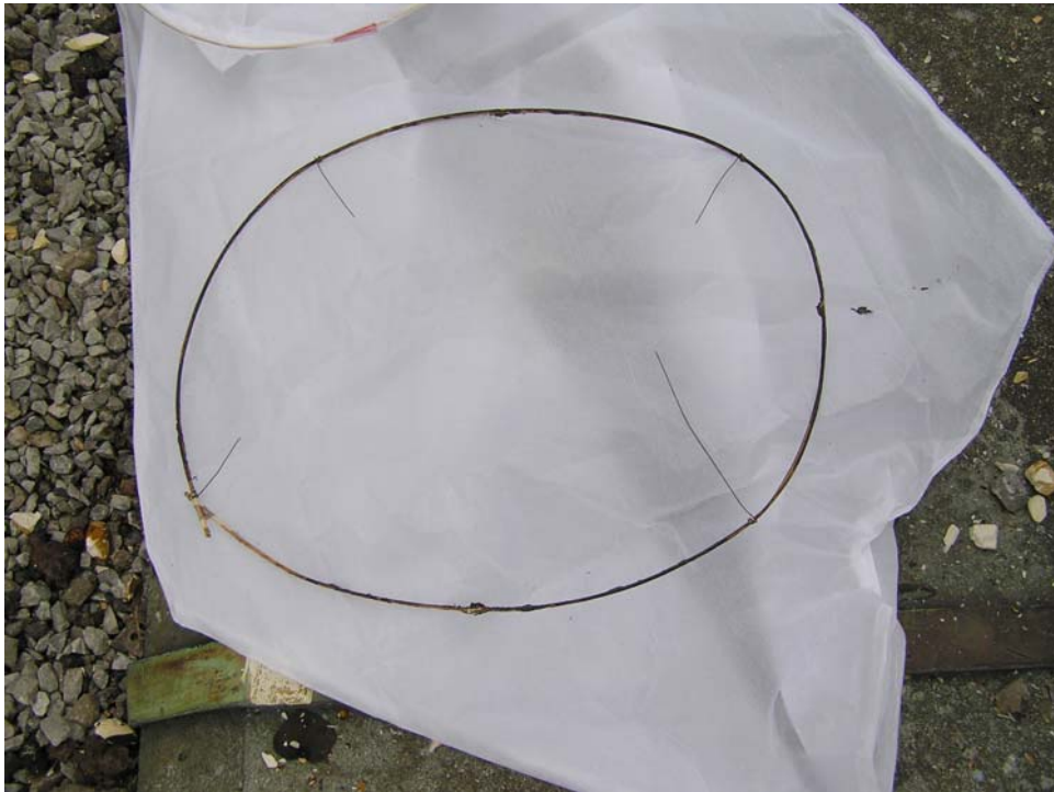
Photograph 1 – Remains of Chinese flying lantern showing the metal ring
