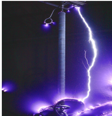
Pictures of AC flashover of field-aged composite insulators (Pictures Courtesy of Manchester University)
