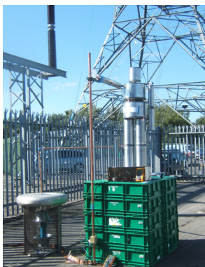
A model man producing microshocks in a substation, and the resulting voltage trace showing discharges.
