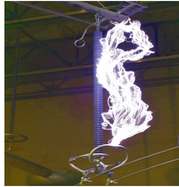
Pictures of AC flashover of field-aged composite insulators (Pictures Courtesy of Manchester University)
