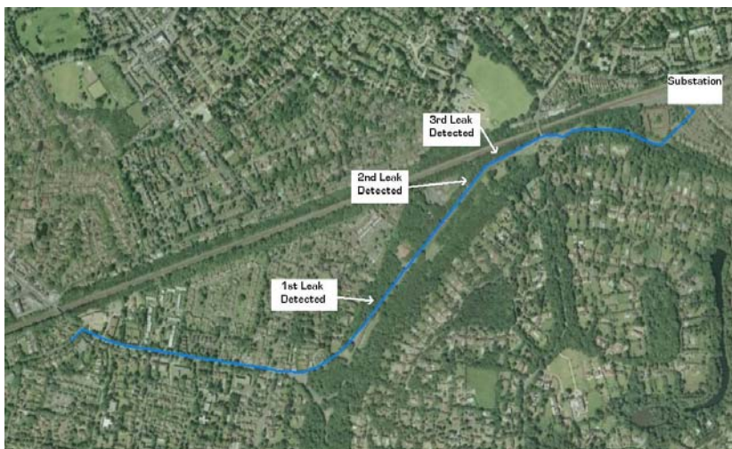
Figure 16 Aerial photograph with FFC and leak locations identified
