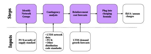
3.5 For the purpose of forecasting future reinforcement the network is broken down into a number of Network Groups. The use of Network Groups for analysis is an important stage in assessing Security of Supply requirements and is consistent with the security of supply standard, P2/6, which also defines the required network capability in terms of the same 'demand groups'. Each Network Group is a part of the distribution system
