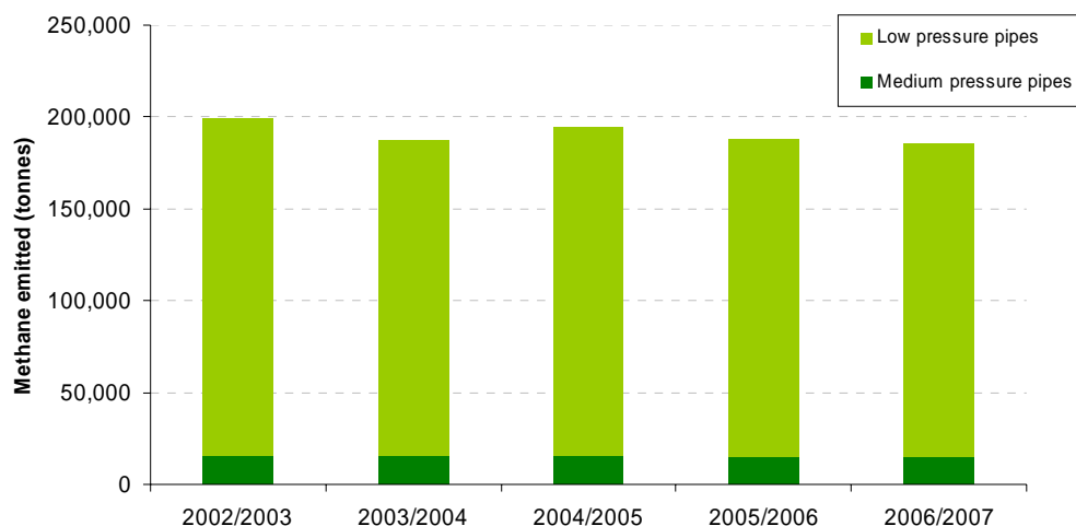
Figure 20: Methane emitted from medium and low pressure pipelines due to leakage
