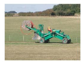
The cable laying plough makes a narrow slit and at the same time several cables or pipes can be placed at the base of this slit up to a maximum depth of 2.0m. As no earth is dug out, the soil structure remains unchanged and the surface is immediately closed so that it returns to its original condition very quickly.
