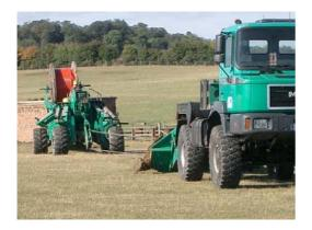
A development of proven cable/pipe laying equipment has produced a system to install multiple power cables quickly, cheaply and with minimal disruption.
