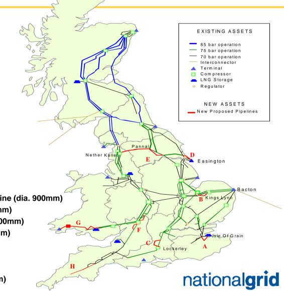
A Isle of Grain to Shorne to Gravesend pipeline (dia. 900mm)
