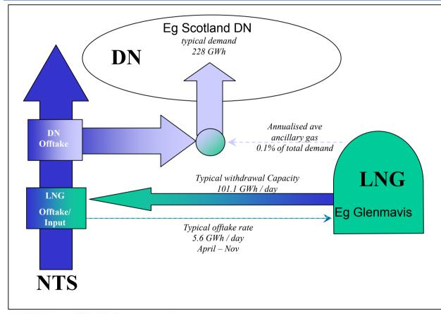
• LNG flows to DN are boil off and reject.
