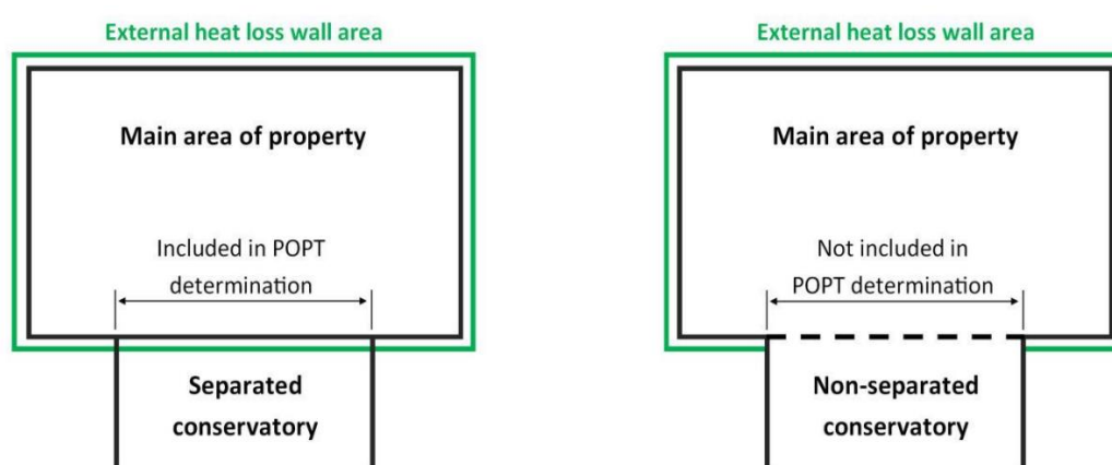
Figure 13: POPT Diagram for Properties with Fully Glazed Conservatories
