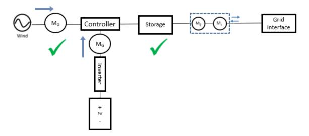
2.46. In this scenario, there is a generation meter after each separate type of renewable generation and before the battery storage. Different technology types on a colocated site would have separate accreditations. Each meter is capable of measuring gross renewable generation from individual technology types. On this basis, in this instance, the requirements for generation payments are met.
