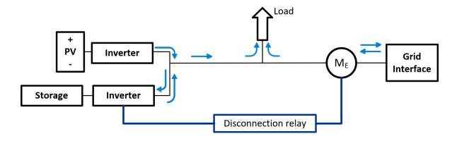
A3.10 The configuration of the site means that the storage can only be charged by electricity generated by the SEG installation. In this example, a disconnection relay
