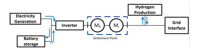
A2.19 In this scenario, electricity battery storage has been co-located with the RO generating station with hydrogen production equipment installed after the metering point. This is not technically a co-location scenario as the generated electricity will pass through the meter before reaching the storage. The metering in place at the settlement point measures the electricity generated.
