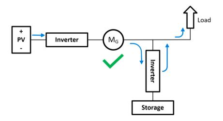
In this off-grid scenario the co-located storage is installed after the generation meter, the generation meter is a meter which is not capable of measuring a net value. The storage can be charged only by electricity generated by the FIT installation. The storage facility is able to help supply the on-site demand.
