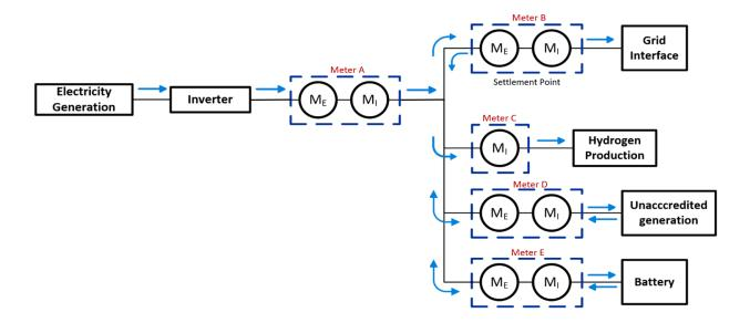
A2.39 In Potential Example 1a, the presence of an import and export meter after the inverter means that eligible generation can be accurately calculated for the accredited station.
