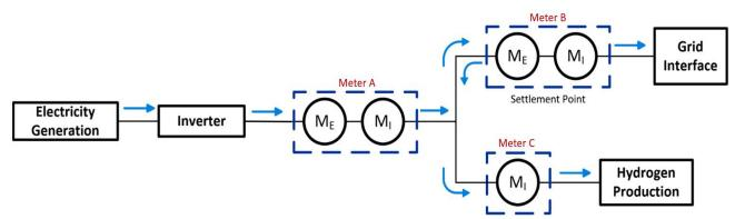
A2.24 In Scenario 5a, three meters allow for the input electricity to be accurately deducted so that ROCs are only issued for eligible electricity generation.
