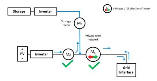
In this scenario, co-located storage has been installed and is supplied by the generating station via a private wire network. The FIT installation and the storage share a bi-directional export meter. The electricity generated by the FIT installation is either supplied to the storage facility or exported to the grid. The storage facility is also able to import electricity from the grid.
