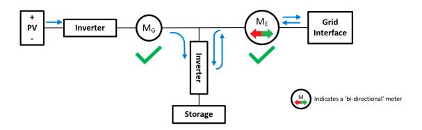
In this scenario the co-located storage is installed after the generation meter, the site is a stand-alone installation and does not have an on-site load (beyond the auxiliary load of the installation). The export meter is a "bi-directional meter", which is capable of measuring a net value. The storage can be charged by both electricity generated by the FIT installation and electricity imported from grid, and can export to the grid.
