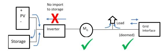
In this scenario, the co-located storage is installed before the generation meter and shares an inverter with the solar PV FIT installation. It is assumed that the requirements to qualify for deemed export are met.<sup>24</sup> Here, the generation meter is capable of measuring output from both the FIT installation and the storage facility.
