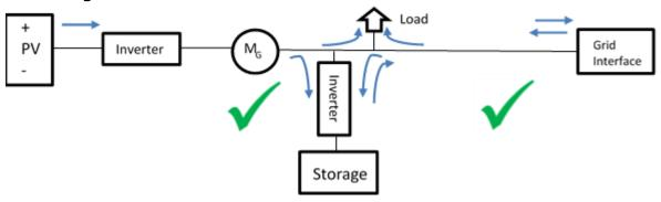
In this scenario the co-located storage is installed after the generation meter. It is assumed that the requirements to qualify for deemed export are met.<sup>21</sup> The storage can be charged by both electricity generated by the FIT installation and electricity imported from the grid. The storage facility is able to supply any on-site demand and can export to the grid.
