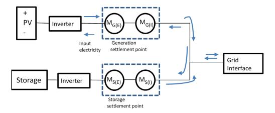
2.28. In this scenario, co-located storage has been installed with the RO generating station, the settlement metering point for the generating station has been relocated, so there are dedicated settlement meters for both the storage facility and the generating station. This may be accomplished by ensuring both the generation and the storage facility have separate meter point administration
