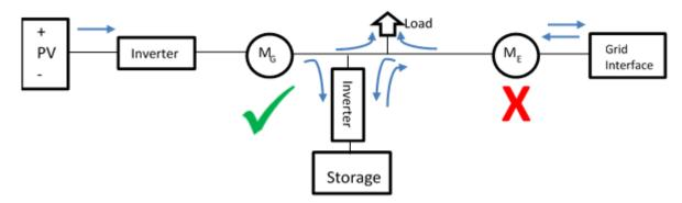
In this scenario the co-located storage is installed after the generation meter. The generation meter and export meter are meters which are not capable of measuring a net value. The storage can be charged by both electricity generated by the FIT installation
