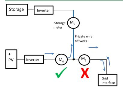
In this scenario, co-located storage has been installed and is supplied by the generating station via a private wire network. The FIT installation and the storage share an export meter. The electricity generated by the FIT installation is either supplied to the storage facility or exported to the grid. The storage facility is also able to import electricity from the grid.
