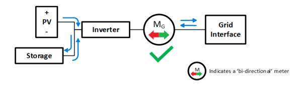
This scenario is the same as 4.4. but it does not have a load output. In this scenario, the co-located storage is installed before the generation meter and shares an inverter with the PV FIT installation. The generation meter is a "bi-directional meter", which is capable of measuring input and output, and calculating and displaying a net value. The storage facility can only be charged by electricity imported from the grid.
