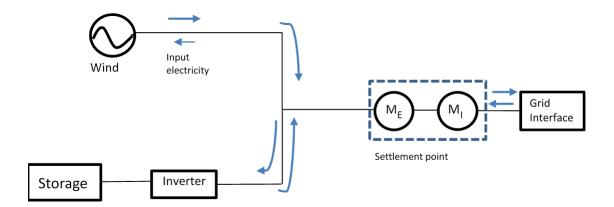
2.22. In this scenario, storage has been co-located with the existing RO generating station. There have been no changes to the metering point previously used, before the storage facility was installed. The storage facility can be charged by electricity produced by the generating station, as well as by electricity imported from the grid that passes through the import meter.
