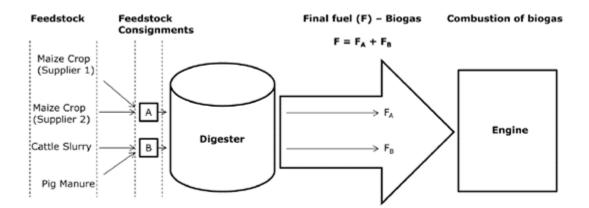
2.46 The resulting final fuel (F), in this case biogas, can then be apportioned according to the consignments of Consignment A and Consignment B.
