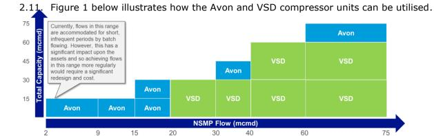
Figure 1 – St Fergus Gas Terminal Compressor Utilisation
