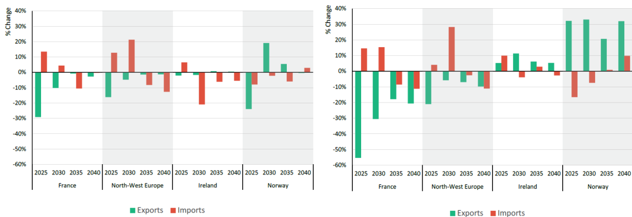
Figure 4.5: Percentage change in scheduled interconnector flows, grouped by landing point region. Zonal relative to national (left) and nodal relative to national (right). LTW NOA7. Source: FTI.
