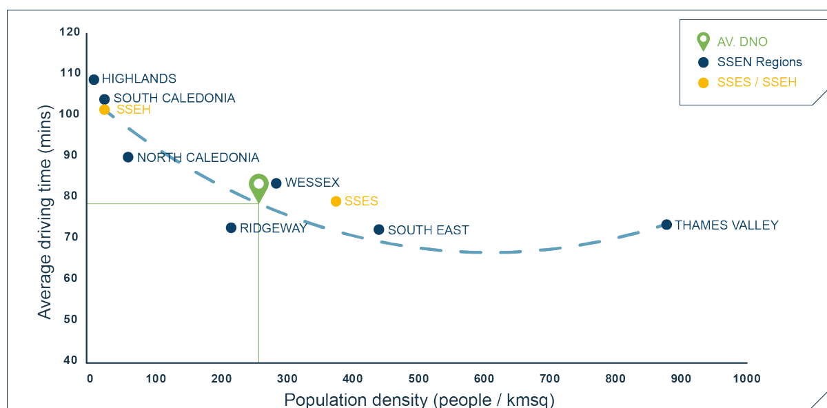
Figure 12: Average driving times plotted against population density for SHEPD and SEPD, and the seven regions within SSEN's network
