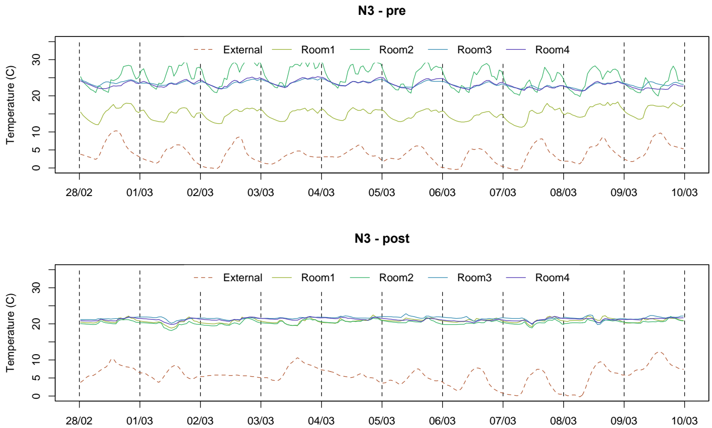
Figure 8: Pre and post retrofit temperatures in Notts 3 over 10 days
