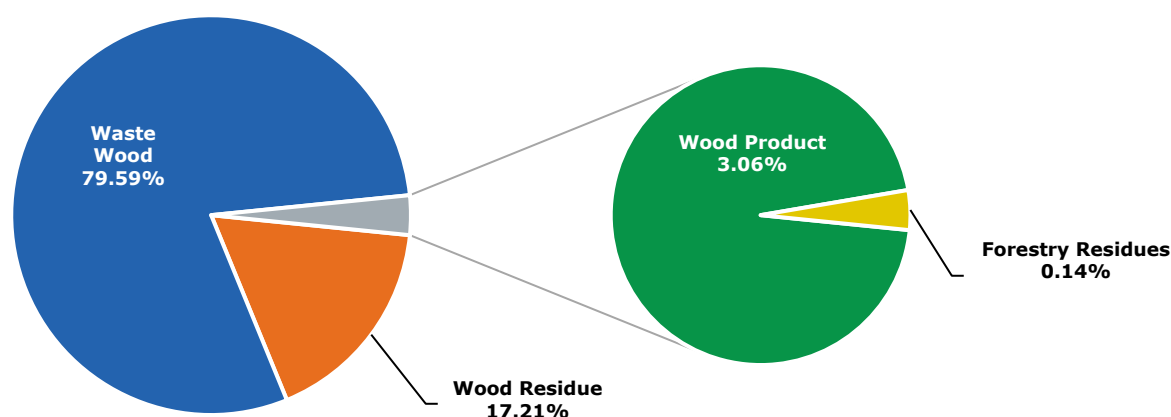
Figure 3.1: Type of feedstocks used (by volume of gas burnt) in gasification stations
