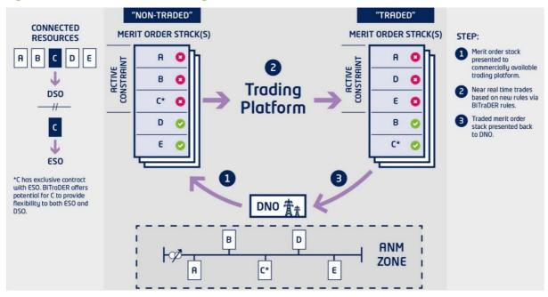
Figure 2.1: BiTraDER Method diagram
