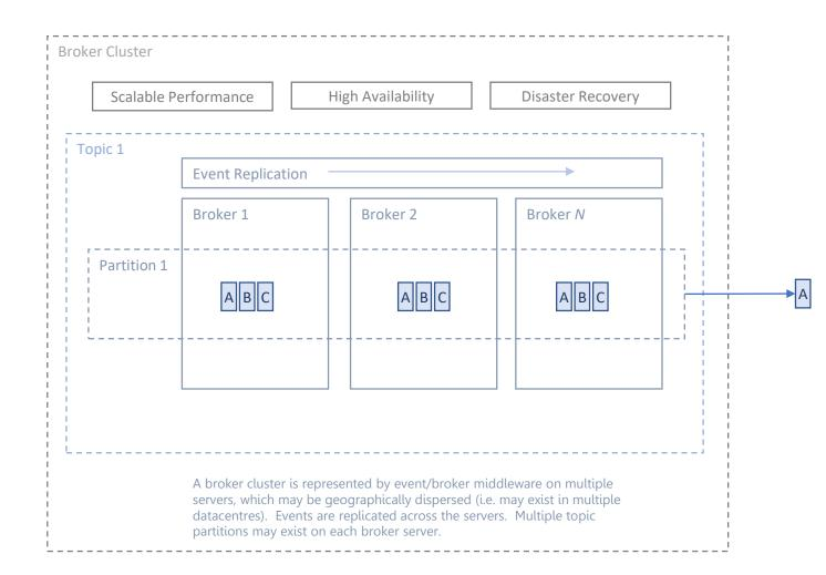
The event backbone utilises clusters of broker servers for high performance, parallelism, fault tolerance and high availability.
