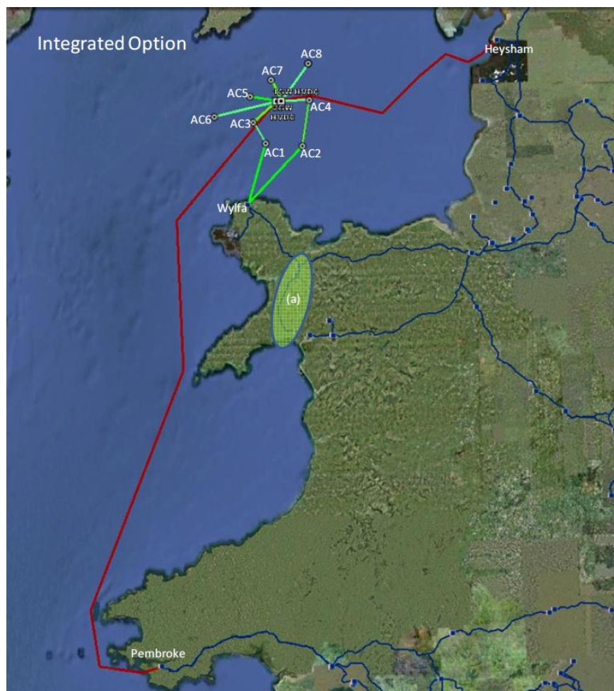
Figure 2 Coordinated development of offshore transmission in the Irish Sea
