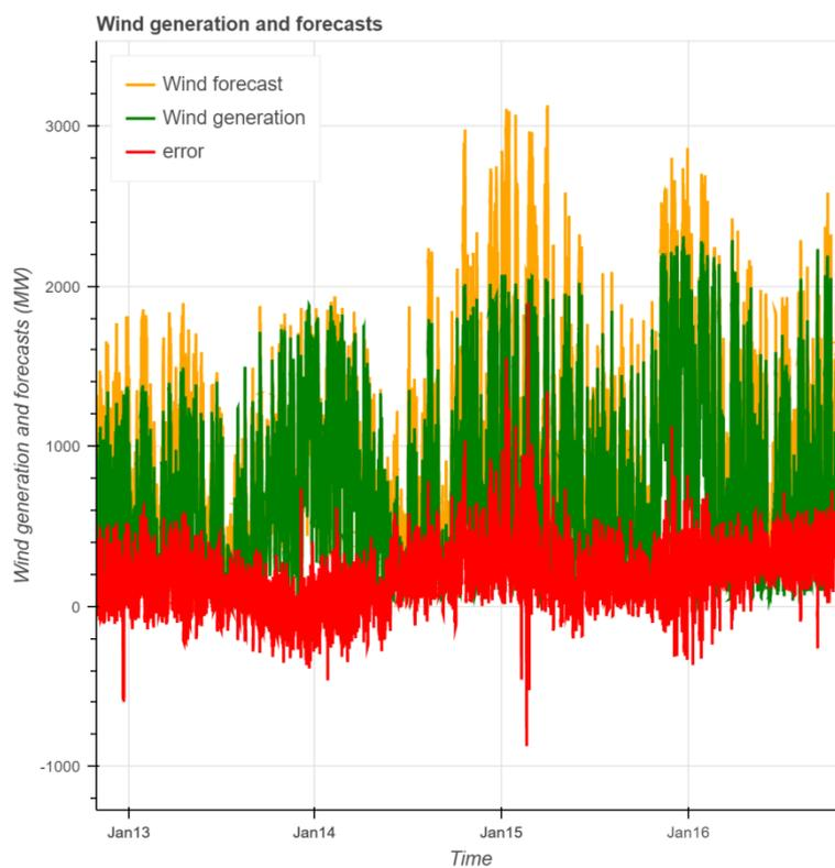
Figure 4 Embedded wind generation forecast and actual wind generated by off-shore and on-shore wind turbines with their signed difference.
