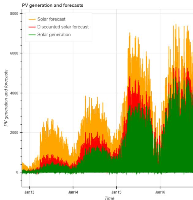
Figure 3 Solar PV forecast generation along with the reduced forecast, where the PV forecast is reduced according to the fraction of capacity of 50kW and above PV installations to the total PV capacity. The green is the total output across all PV sites in the dataset. The x-axis is time, and the y-axis is in units of MW.
