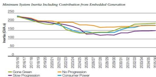
Figure 1 displays the future minimum system inertia including the contribution of embedded generation for National Grid's four future energy scenarios [National Grid, System Operability Framework 2015].
