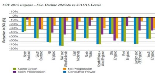
Figure 2 illustrates the future decline in short circuit level expected from 2015/16 to 2025/26 and states the level in South Scotland could fall 50% under two of National Grid's four future energy scenarios [National Grid, System Operability Framework 2015].
