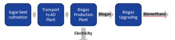
This first figure shows the 'biogas production plant' as a black-box, from which exit both biogas and electricity. In this view, there is no heat co-produced (assuming all heat is utilised on site); the only coproduct is electricity. Following the approach set out in section 4.2.2.3, upstream GHG emissions should then be allocated between biogas and electricity based on their energy contents.
