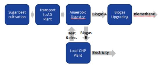
In this second figure, the 'biogas production plant' is deconstructed into 2 separate components:
