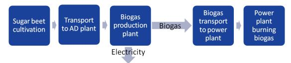
This first figure shows the biogas production plant as a black-box, from which exit both biogas and electricity. In this view, there is no heat co-produced; the only co-product is electricity. Following the ROO, upstream GHG emissions should then be allocated between biogas and electricity based on their energy contents.
