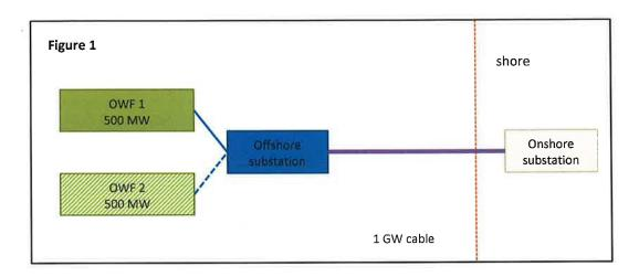
While OWF 1 will have an oversized connection (1 GW compared to the 500 MW size of the wind farm) before OWF 2 is completed, it will still have a single point of failure and no benefit in terms of increased redundancy. The benefit of the anticipatory investment is mainly in terms of reducing the total CAPEX of the transmission assets, rather than increased redundancy for the generator.
