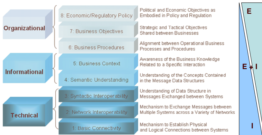
GridWise Architecture Council - smart grid interoperability framework
