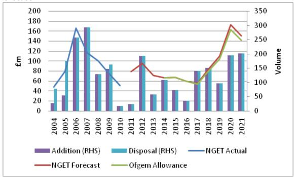
Figure 5.5 - Comparison of overhead line replacement performance and forecast
