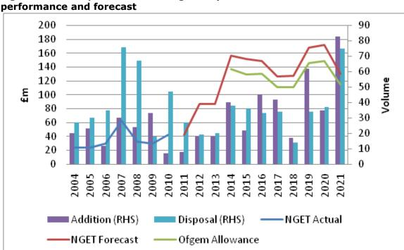
Figure 5.4 - Comparison of switchgear replacement & refurbishment performance and forecast
