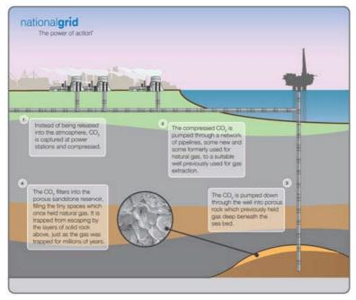
Figure 17 Schematic of National Grid's Carbon Transport and Storage project
