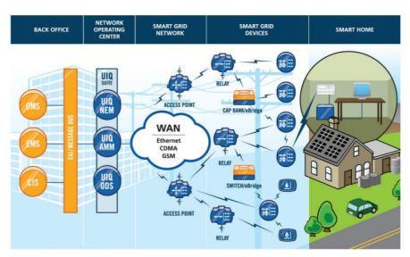
Figure 7 Illustration of the communication layers of the Smart Miami project
