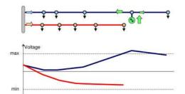
Figure 12 Voltage on a feeder with load only (red trace) against voltage on a feeder with generation (blue trace)
