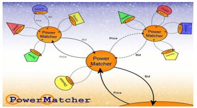
Figure 5 Relationships between the elements controlled by PowerMatcher
