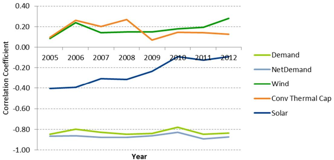
**Figure 30 – Correlations of capacity margins with system parameters (Spain, without IC Flows)**
