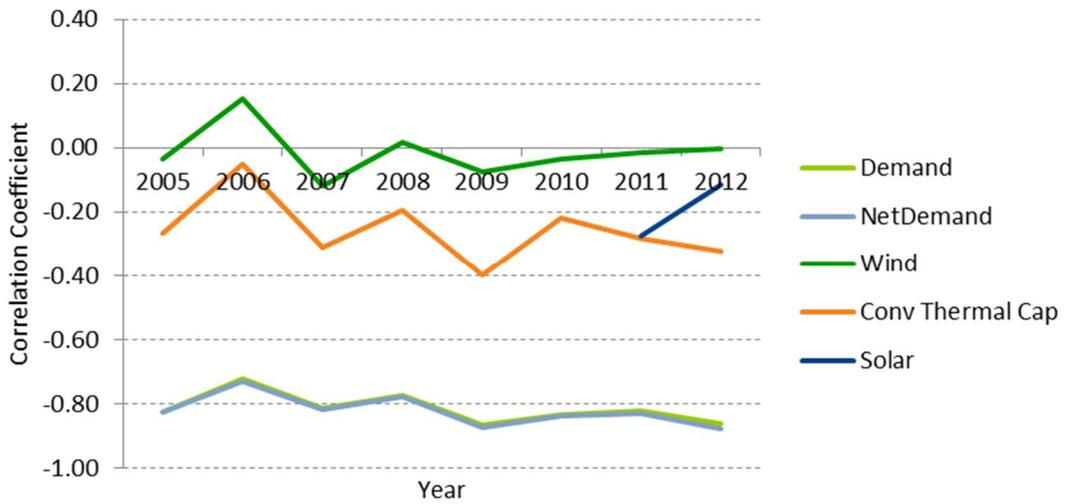
**Figure 27 – Correlations of capacity margins with system parameters (Ireland, without IC Flows)**
