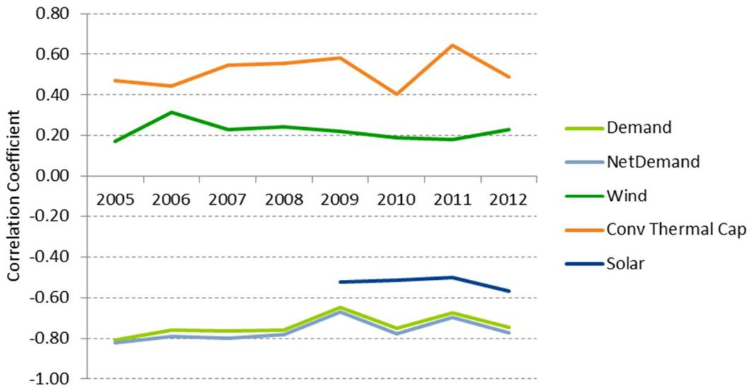
**Figure 29 – Correlations of capacity margins with system parameters (Germany, without IC Flows)**
