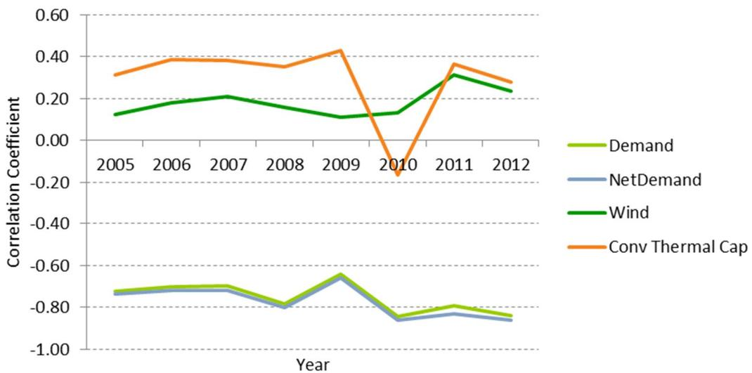
**Figure 28 – Correlations of capacity margins with system parameters (The Netherlands, without IC Flows)**
