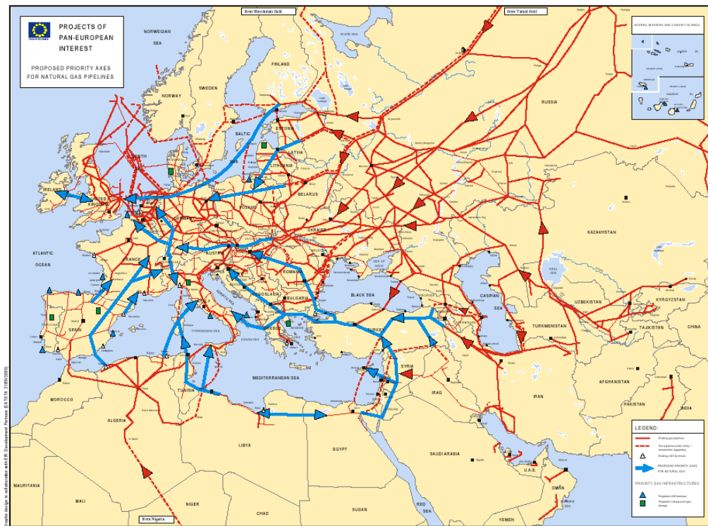
Source : "Projects of Pan European Interests" : Map presented to the Euro-Mediterranean Ministerial Meeting of May 2003 to illustrate existing pipeline interconnectivity and proposed priority axes for future natural gas flows.
